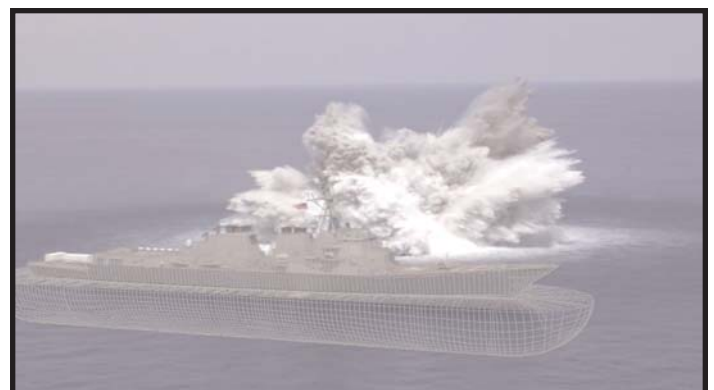
Finite Element Mesh Overlay of the Coupled Ship Structure and Fluid Volume for DDG-81 Shock Trial
