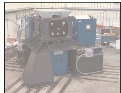
Figure 4: NAVSEA Keyport's 3-Axis Electro-Dynamic Vibration Test System
