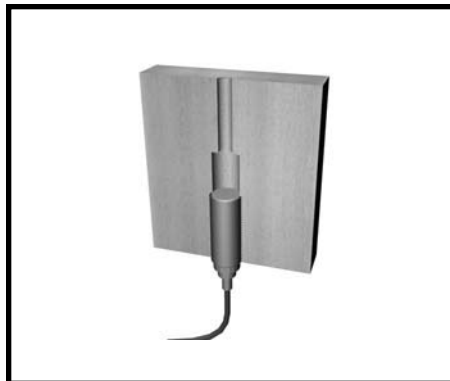
Figure 8: Pressure Transducer with Tubing and Associated Volume Interconnect
