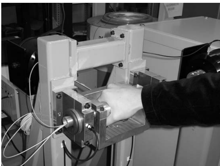
Fig. 1 - Patient grasping special Test Handle with embedded Force & G sensors
